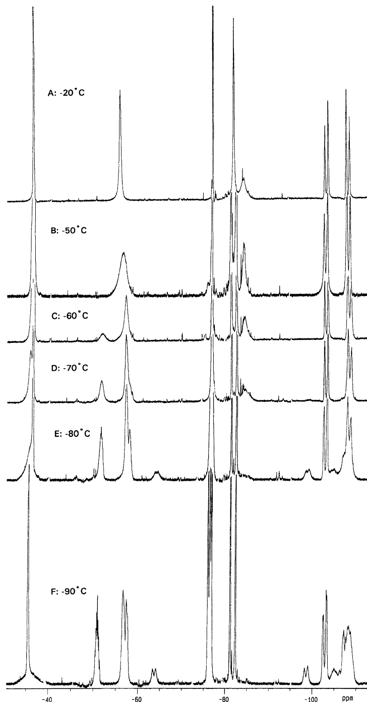
Fig. 3. ^{19}\text{F} -NMR low temperature spectra of the carbanion in the temperature range up to -90^\circ\text{C} .
